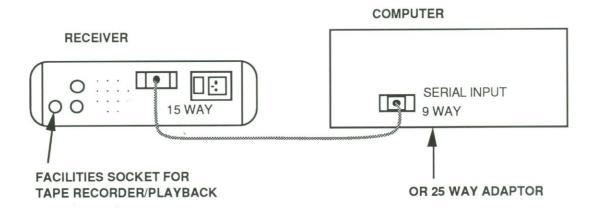
The DIN connector can be plugged into the facilities socket if connection to a cassette recorder is required. The cable is coded as follows:-
